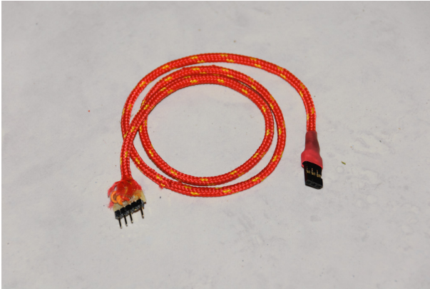
Fig. 4 - the signal cable, protected with a sleeve, with the separation connector (still “naked”) at one end, and a servo plug CA-bonded to the sleeve and covered in heat shrink tubing at the other end
