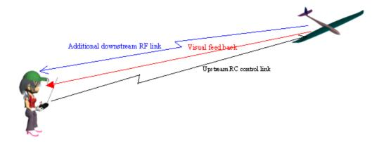
Fig 2 – Improved feed back loop with addition RF link
